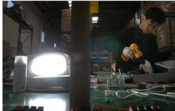
Mark Moon, with US Lighting Tech in Signal Hill, assembles a 100-watt street light. The process takes only about 20 minutes, as the majority of the parts he uses are shipped to the company intact from China and Korea. (Diandra Jay/Staff Photographer)
